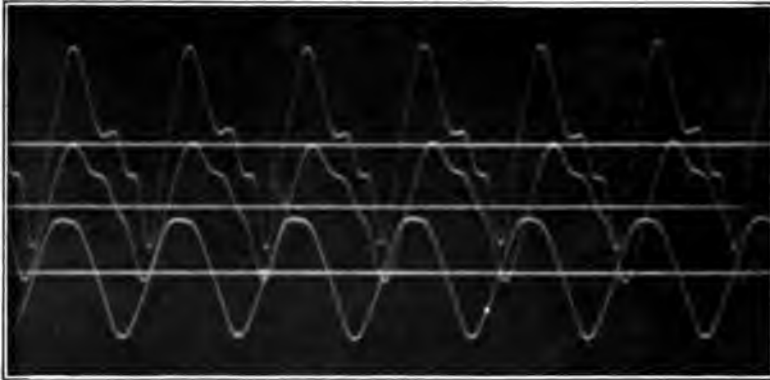
FIG. 139. Three photographs of the tone of a flute, played p , mf , and f .
